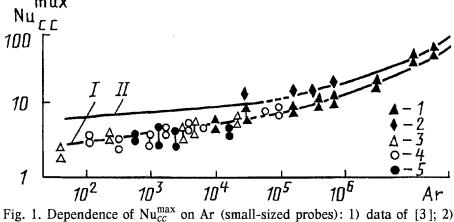
Fig. 1. Dependence of  $Nu_{cc}^{cc}$  on Ar (small-sized probes): 1) data of [3]; 2) [1], D/d = 1; 3) [4]; 4) [5]; 5) [2]; I) calculation by Eq. (7); II) calculation by Eq. (7) for D/d = 1.
