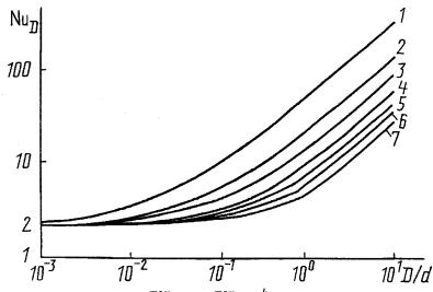
Fig. 2. Dependence of  $(Nu_{cc}^{max})_D = \alpha_{cc}^{max} D/\lambda_f^k$  on the ratio D/d for different values of Ar: 1–7) Ar = 10<sup>7</sup>, 10<sup>6</sup>, 10<sup>5</sup>, 10<sup>4</sup>, 10<sup>3</sup>, 10<sup>2</sup>, 10<sup>1</sup>, respectively (calculation by Eq. (8)).
